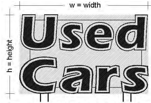
Calculating Area of a Sign where Copy Exceeds Sign Area = (height of copy) x (width of copy)
